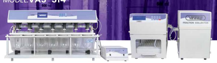
A multi-syringe dosing pump is designed specifically for parallel sample withdrawal and dosage of media from a dissolution bath into open vials inside a fraction collector. It operates with multiple valve system. It is equipped with replaceable high precision glass syringes. The syringe dosing pump is available as additional part of the offline dissolution system packages.
